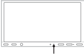
Bluetooth signal indicator: Lights up when the Bluetooth signal is on.
